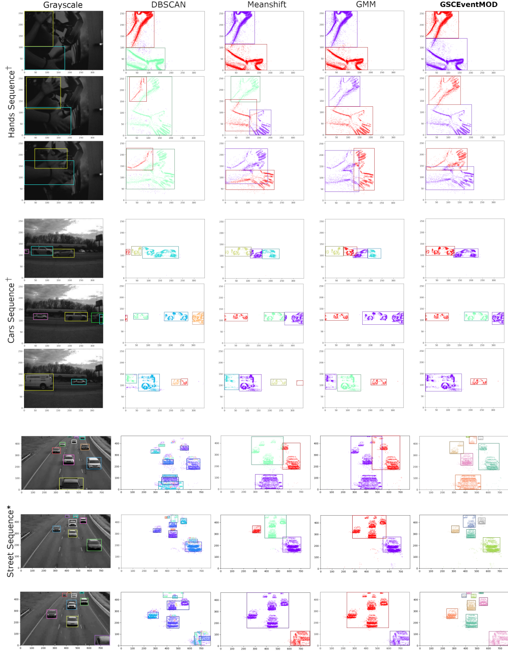
Figure 4: Visual results for GSCEventMOD and other SOTA methods on the DistSurf [2] (marked with †) and the synthetic dataset (marked with *). We show that our method performs significantly better than the other compared methods (best viewed in color).
